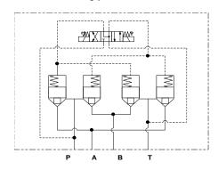
• With 3x2 Solenoid independent logic control : X4 Type
